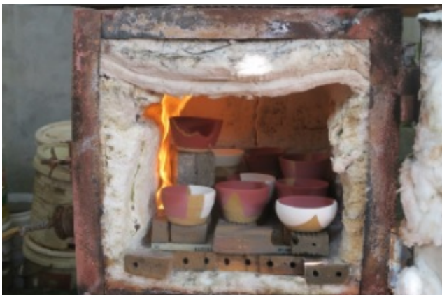
A gas kiln with raw ceramics is set to be fired. Photo: Nicolò Tissier
